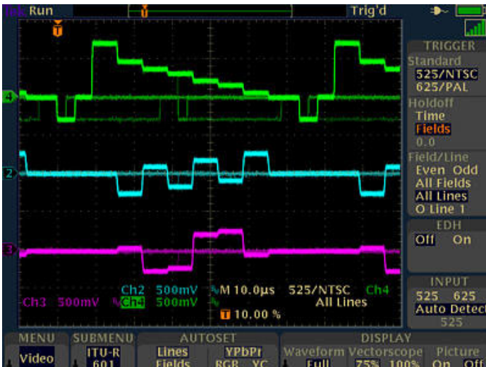
Trace and identify ITU-R BT.601 video signals with the TDS3SDI 601 Serial Digital Video Module.
